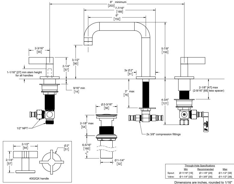
[Dimensions in brackets are mm, rounded to 1mm]
