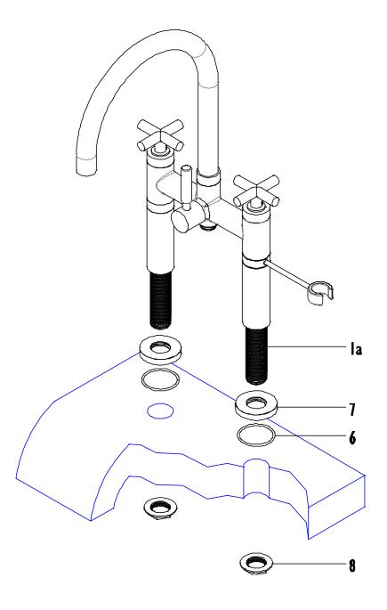
**WARNING:** When soldering or use of FLAME on leg SHANK (1a), it is the responsibility of the installer to take proper steps to prevent over heating of the leg SHANK (1a) to prevent damage to sealed joint between LEG (1) and leg SHANK (1a). All soldering shall be a minimum of 4" away from joint
