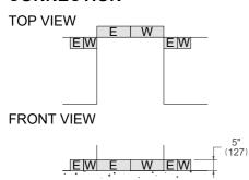
A properly-grounded, horizontally-mounted electrical receptacle should be installed according to this drawing.
