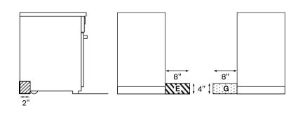
Installation clearance available behind range Electrical Installation Location Gas Installation
