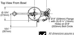
All dimensions assume standard thread engagement. Variations in manufacturing allow for +/- ½" (3mm) per threaded joint. To find the tolerance of a dimension, add the number of thread joints in between a dimension and multiply it by ½" (3mm).
