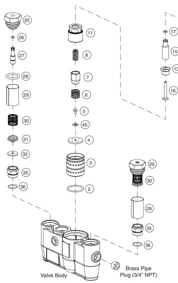
NOTICE! Some threaded joints are assembled using high strength thread lock and may require the use of heat to loosen the connection. Use caution to not damage o-rings or other components.
