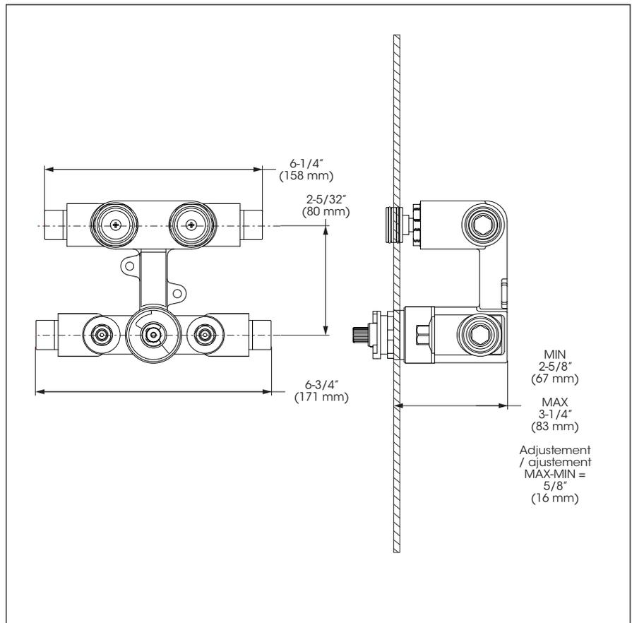
Valve - Rough-In // Thermostatic 2-way Diverter Valve
