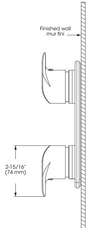
Valve – Trim for Thermostatic 3-way Diverter Valve
