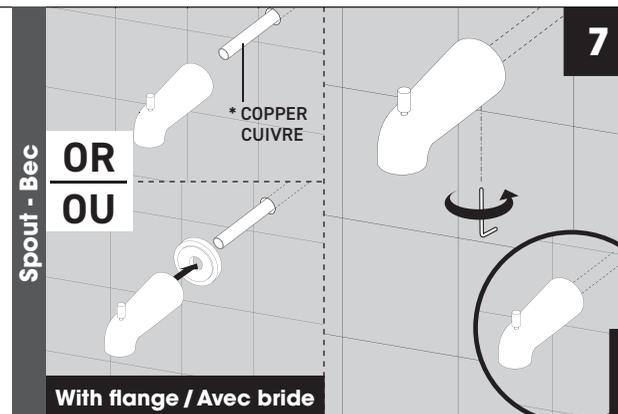
\* We insist on using copper pipe to connect the valve to the spout and to the shower head. PEX pipe adaptors can cause flow restriction, thus creating a backflow to the showerhead.
