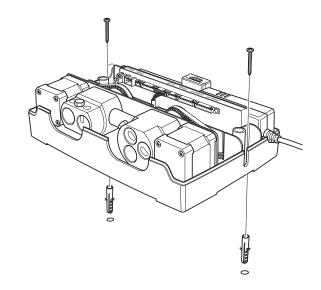
If required, use the supplied template (provided in the install guide) to mark the position of the control mixer fixing holes in the selected location.
