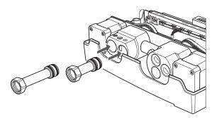
Fully insert the inlet connectors into the inlet valves (one long and one short connector).
