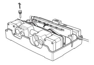
Remove the inlet connectors' retaining bolt.
