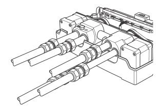
Attach the supplied NPT adaptor pipework to the outlet connectors. Make a note of which pipe goes to which outlet.
