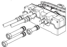
Fully insert the outlet connectors into the outlet valves (one long and one short connector).
