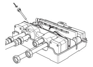
Re-insert the outlet connectors retaining bolt.
