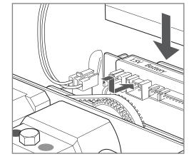
Connect the battery cable to the "Battery for battery back-up" connection and place the battery in the compartment.
