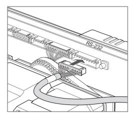
Connect the data cable from the Vision Wheel interface connection in the "RS-232" port in the control box.
