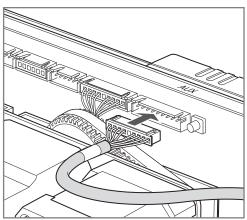
Connect the data cable from the flow volume/ divertor control to the "dual wheel" connection in the "AUX" port in the control box.
