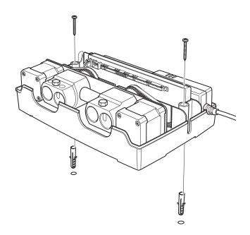
If required, use the supplie template to mark the position of the control mixer fixing holes in the selected location.
