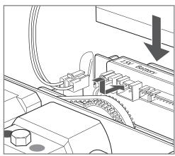
Connect the battery cable to the "Battery for battery back-up" connection and place the battery in the compartment.
