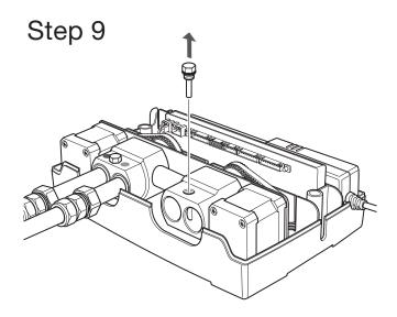
Remove the outlet connectors' retaining bolt.
