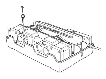
Remove the inlet connectors' retaining bolt.
