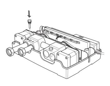
Re-insert the inlet connectors retaining bolt.
