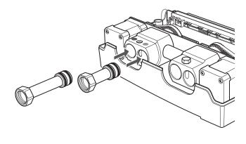
Fully insert the inlet connectors into the inlet valves (one long and one short connector).
