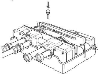
Re-insert the outlet connectors retaining bolt.
