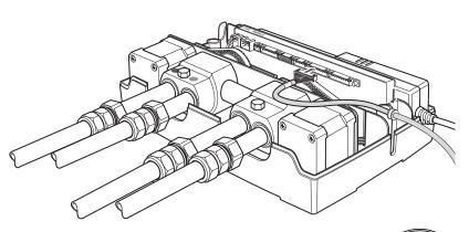
Connect the data cable from the on-off/temperature control to the 'TLI' port in the control box.
