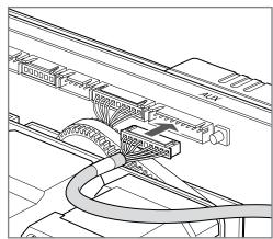
Connect the data cable from the flow volume/ divertor control to the "dual wheel" connection in the "AUX" port in the control box.
