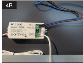
Connect cable (3) blue / (4) brown from the transformer (B) to the infrared switch (C)
