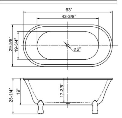
L: 63" W: 29-5%" H: 25-1/4" Water depth: 17-3%" to top of tub The following is recommended for ATDN63LP tubs: •Faucets: part #4602, 4022 or 4025 •Rigid, freestanding supplies: part #4502 •Rigid, freestanding supplies: part #4502 •Freestanding filler: part #7901, 7918 or 7934 (Does not need bath supplies) •Leg tub drain: part #5599LT or 5599TS
