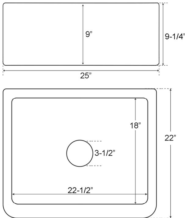
Dimensions of fixture are nominal and may vary within the range of tolerances established by ANSI Standard A112.19.2. Dimensions and specifications subject to change without notice.
