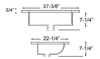
Dimensions of fixture are nominal and may vary within the range of tolerances established by ASME Standard A112.19.2.2013 Dimensions and specifications subject to change without notice.
