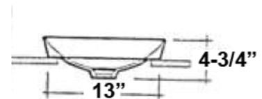
Dimensions of fixture are nominal and may vary within the range of tolerances established by ASME Standard A112.19.2.2018. Dimensions and specifications subject to change without notice.
