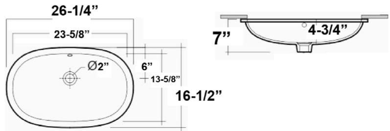
Dimensions of fixture are nominal and may vary within the range of tolerances established by ASMEI Standard A112.19.2. Dimensions and specifications subject to change without notice.
