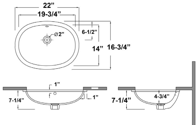
Dimensions of fixture are nominal and may vary within the range of tolerances established by ASMEI Standard A112.19.2. Dimensions and specifications subject to change without notice.
