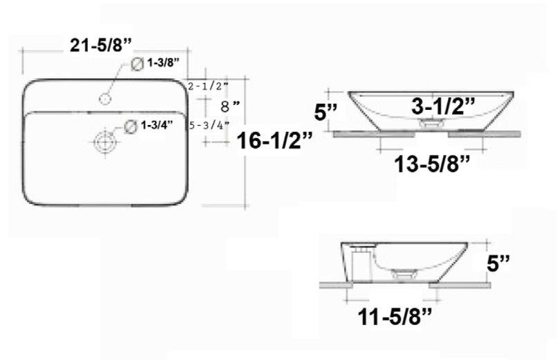
Dimensions of fixture are nominal and may vary within the range of tolerances established by AMSE Standard A112.19.2.2018 Dimensions and specifications subject to change without notice.
