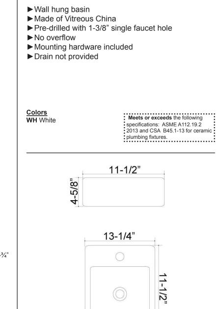
Dimensions of fixture are nominal and may vary within the range of tolerances established by ASME Standard A112.19.2.2013 Dimensions and specifications subject to change without notice.
