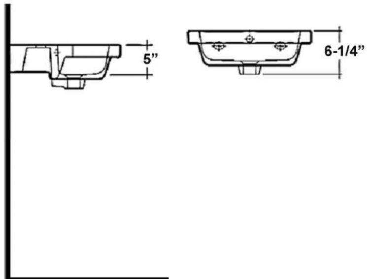
Dimensions of fixture are nominal and may vary within the range of tolerances established by ANSI Standard A112.19.2. Dimensions and specifications subject to change without notice.
