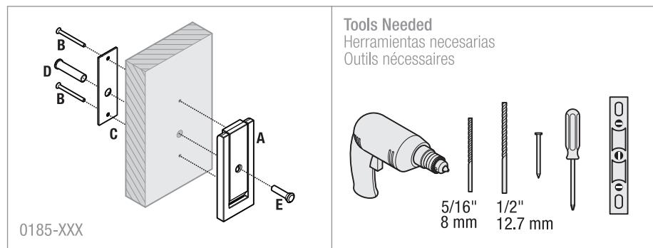
**1** Center template on EXTERIOR side of door. Ensure template is level, and mark holes.
