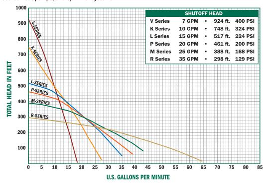
NOTE: Performance shown does not include friction loss in drop pipe (for flow rates above 25 GPM, larger drop pipe is recommended.)
