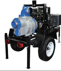
The A.Y. McDonald engine driven trash pumps are constructed of heavy duty sand cast aluminum with cast iron and stainless steel internal parts for wear resistance, and durability. Built-in slide mechanism features nylon and powder coated steel components that permit servicing, repairing, and cleaning entire pump without removing hoses or pump components from trailer.
