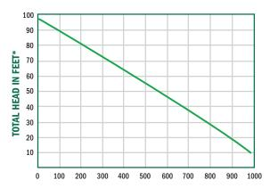
**CAPACITY IN US GALLONS PER MINUTE @ 3600 RPM** \*CONVERT TO PSI, DIVIDE BY 2.31 | LIQUID WATER SPECIFIC GRAVITY 1.0
