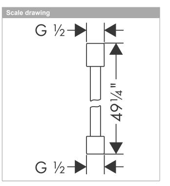
**AXOR Starck** Techniflex Hose with Cylindrical Nut, 49"Finish: polished gold opticPart no. : 28 Part no. : 28282990
