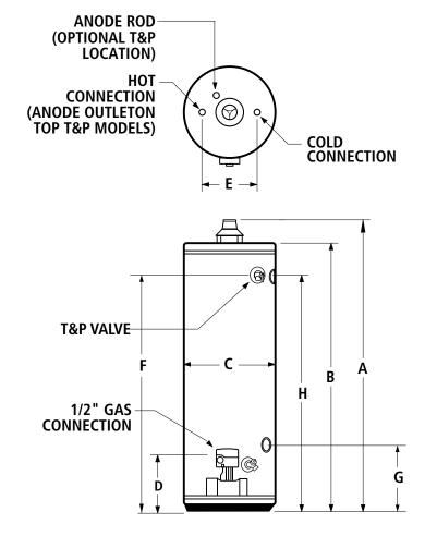
**Maximum Hydrostatic Working Pressure: 150 PSI**
