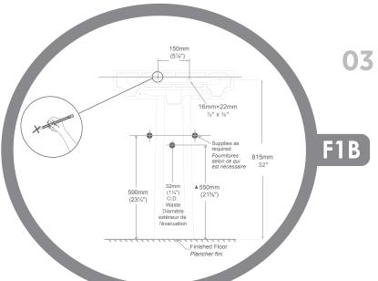
Place the pedestal basin on the pedestal leg and move into the desired position against the wall. Make sure that the pedestal basin is leveled on the pedestal leg. With a pencil, mark the location of the pedestal basin support holes on the wall. (F 1A & 1B)
