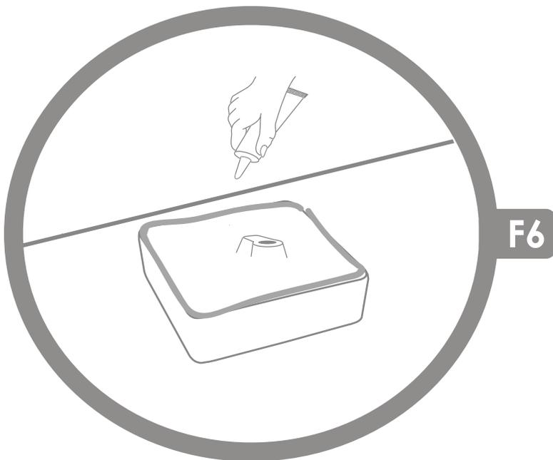
**06** Apply silicone or plumber's putty to the underside outer rim of the vessel sink. Then, secure vessel firmly down and tighten drain assembly under the vanity top. Trim any excess silicone or plumber's putty off. (F6)
