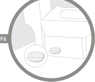
Turn on supply valve and allow tank to fill until float rises to shutoff position. Then place the tank lid on top of the tank.
