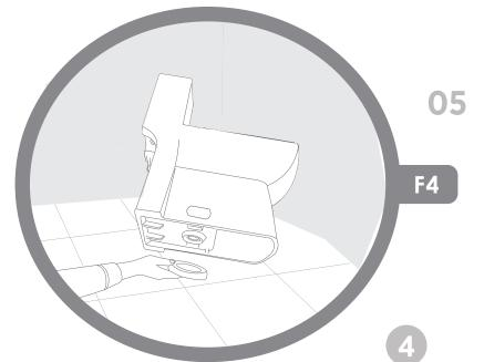
Turn the toilet bowl side ways onto a soft surface to avoid scratches on the finish. Place a new wax ring (not included) around the waste flange of the toilet
