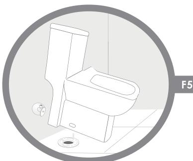
Lower the toilet onto the floor bolts, so the floor bolts project through the mounting holes in the base of the toilet (F5). Using a rocking motion, press the bowl down to position the toilet onto the flange and create a seal with the wax ring.
