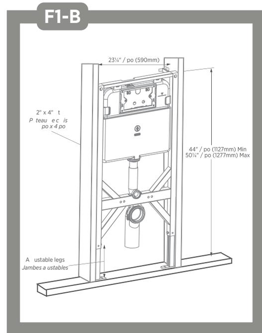
**01** Position the concealed cistern and carrier system into the wall as per the installation instructions. Please follow (F1A) if installing directly onto a concrete wall; follow (F1B) if you are installing using in-wall studs.
