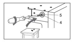
13. On the opposite side from the top hinge, attach the cap (5) using the screw (4).
