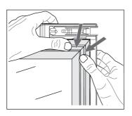
6. Carefully press the gasket back into the groove in the door.
