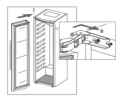
Hang the door onto the screws (2) at the top and bottom and slide it in the direction indicated by the arrow (a).
