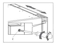
Close the door, then rotate the screw (2) at the top and bottom to adjust the door position.
