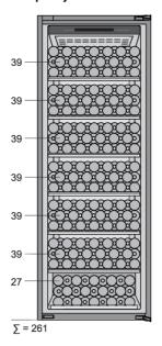
The basic appliance configuration allows storing up to 261 Bordeaux bottles.
