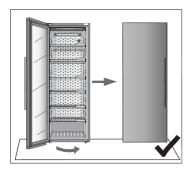
Close the door and make sure it is aligned with the housing. The housing side and the edge of the door should be parallel.
