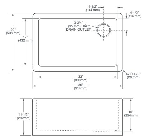
NOTES: \* DIMENSIONS SHOWN FOR LOCATION OF SUPPLIES AND "P" TRAP ARE SUGGESTED. FITTINGS NOT INCLUDED WITH FIXTURE AND MUST BE ORDERED SEPARATELY. SEALING COMPOUND SUPPLIED BY OTHERS.
