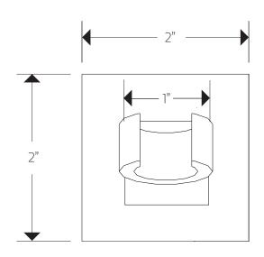
There is a set screw in the bottom face of the escutcheon to secure to the wall bracket
