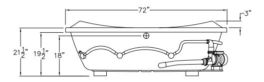
RNRIO 7242 TO DI ACRYLIC FACED DROP IN BATHTUB. CONFIGURED WITH 4 JET WHIRLPOOL SYSTEM, FOOT JETS, PUMP/MOTOR, ON OFF CONTROL, AND CENTER DRAIN.
