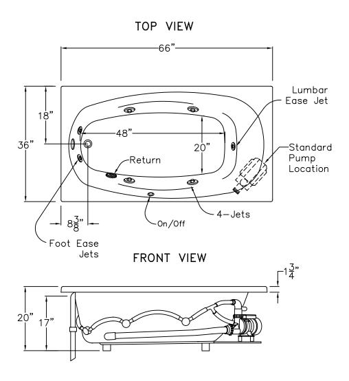
RN 6636 TO DI ACRYLIC FACED DROP IN BATHTUB. CONFIGURED WITH 4 WHIRLPOOL JETS, LUMBAR JET, 2 FOOT JETS, PUMP/MOTOR, AND ON OFF CONTROL.
