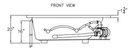
RN 6032 TO DROP IN ACRYLIC WHIRLPOOL. TUB IS CONFIGURED WITH 6 JET WHIRLPOOL SYSTEM, PUMP/MOTOR AND ON/OFF CONTROL.
