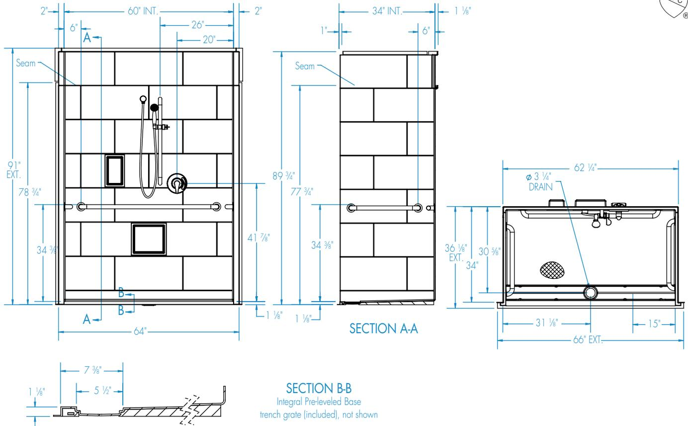
**FEATURES** lbs Dimensional Tolerance  $\pm \frac{3}{16}$ ". Dimensions needed for site preparation should be measured from the unit. Manufacturer assumes no responsibility for preparatory work.
