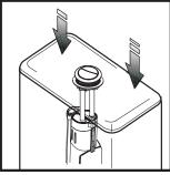
Adjust the direction of the push button. Be sure the full flush Button toward the full flush Touch piece.
