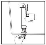
3) installing Fill Valve: To install into tank, remove locknut and slide Fill Valve into the hole in tank. Next, position Fill valve to desired position and tighten the locknut.
