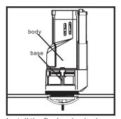
Install the flush valve body on the base again, rotate it to a proper position and lock.
