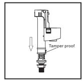
2) After adjusting height of Fill valve, rotate the upper shank counter clockwiseto lock into lower shank. Next. push down
