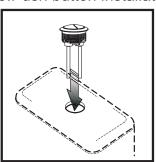
Cut the adjustment rod to a proper length, put the push button into the hole.
