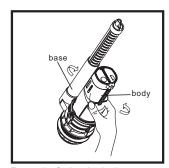
Rotate the flush valve body separate the body from base as shown in the
