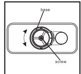
Install the flush valve base into the outlet to make the "U" clasp can clip on the tank properly. Rotate the base to choose proper angleand lock the screw.
