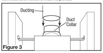
Ensure duct joints and exterior penetrations are sealed with caulk or other similar material
