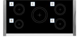
A: 1,850 watts with 3,000 watt Boost: 7" dia. B: 1,400 watts with 2,200 watt Boost: 6" dia. C: 2,300 watts with 3,700 watt Boost: 10" dia. D: 1,850 watts with 3,000 watt Boost: 7" dia. E: 1,850 watts with 3,000 watt Boost: 7" dia.
