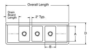
3 Compartment Sink with 2 drainboards Shown
