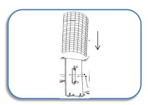
Attach the glass panel to the fixture housing by sliding the glass into the glass guides found on either side of the fixture housing.
